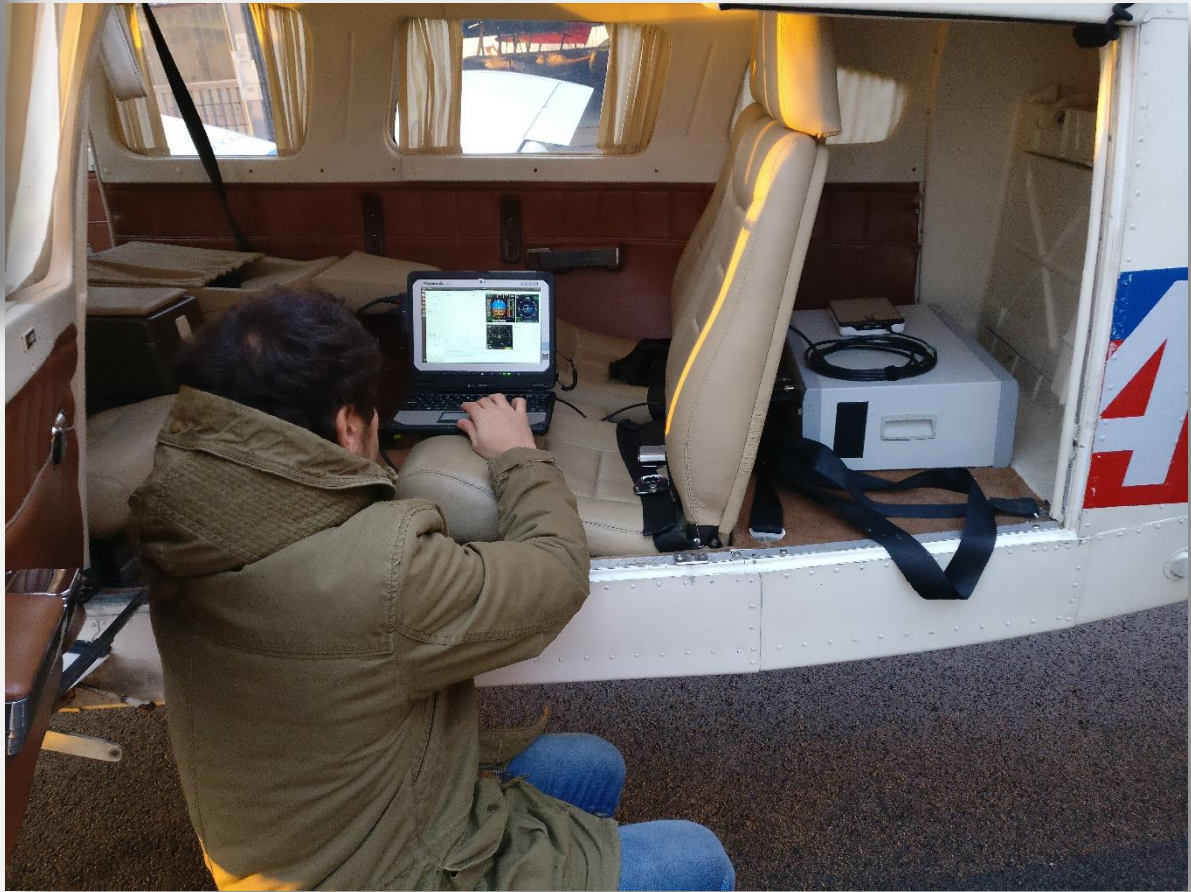
Installation of PILDO data recording equipment components
